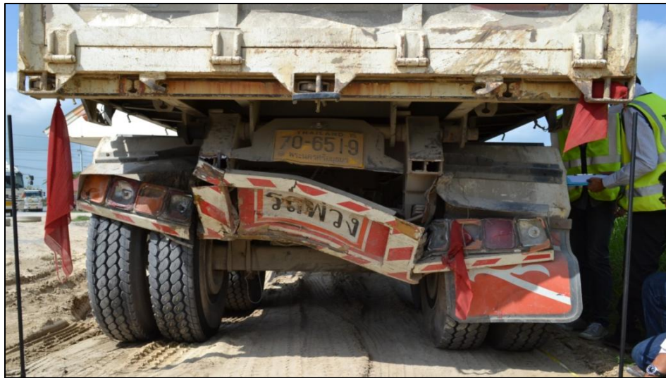
Figure 9 Damages of Trailer-truck
