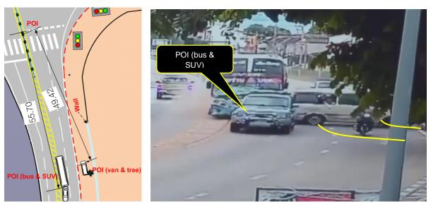
Figure 29 POI between bus and van, and rotation of van before impact
