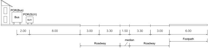
Figure 25 Road section at POR of bus and SUV
