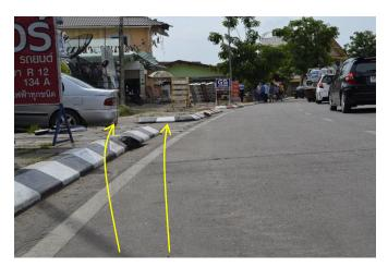
Figure 34 Tire marks showing the bus running off the road
