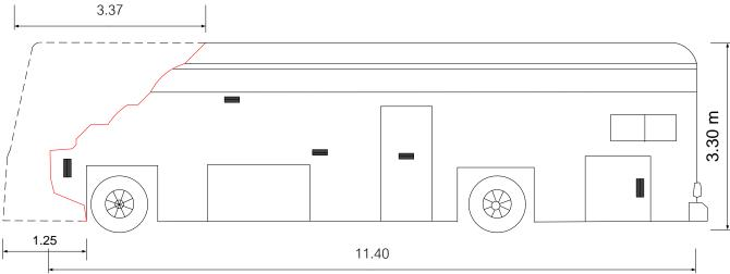
Figure 8 Deformation on the front part of the bus (left side view)
