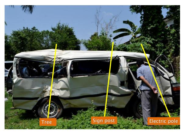
Figure 16 Deformation in right side of van
