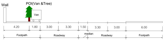
Figure 24 Cross section of the road at POI between Van and roadside tree
