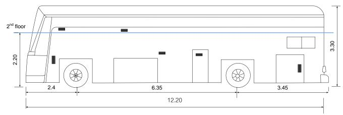
Figure 4 Dimensions of the bus
