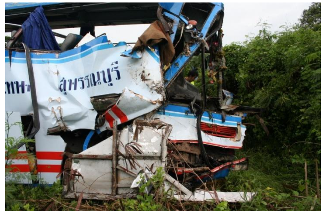
Figure 3-4: Frontal Deformation of the Bus
