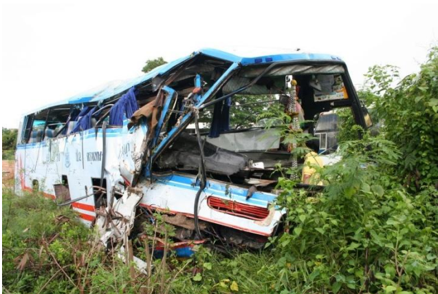
Figure 3-4: Frontal Deformation of the Bus
