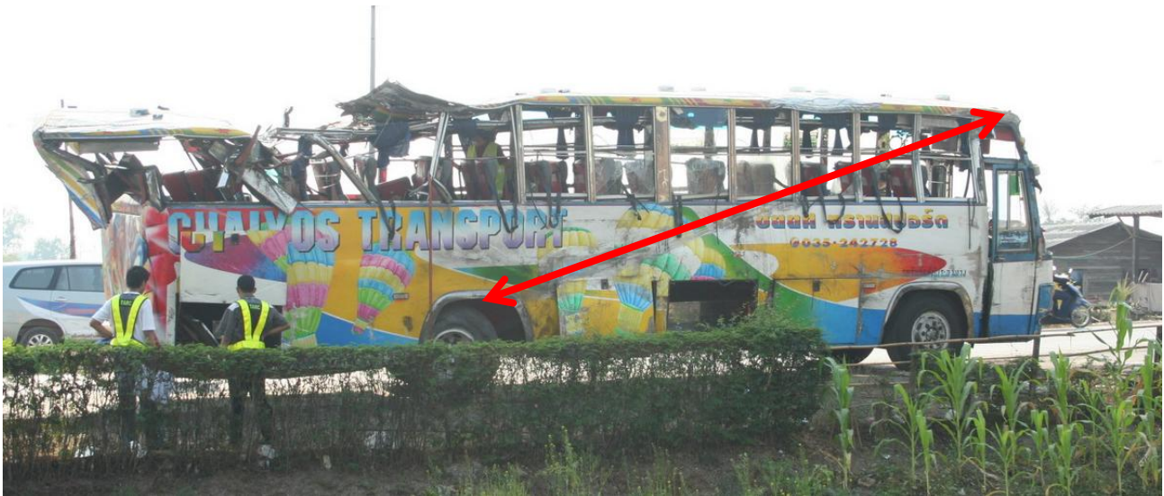
Figure 3-7: Damage Pattern on the Right
